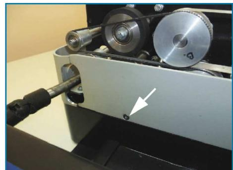
9. Remove the two screws on the inside.
