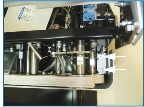
11. Remove the two screws on the inside.
