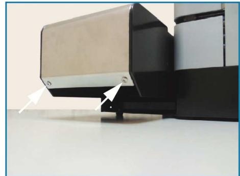
2. Turn the tension bolts to adjust the tension.
