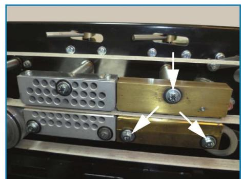
7. Loosen the hex socket bolt at the back of the heating block.
